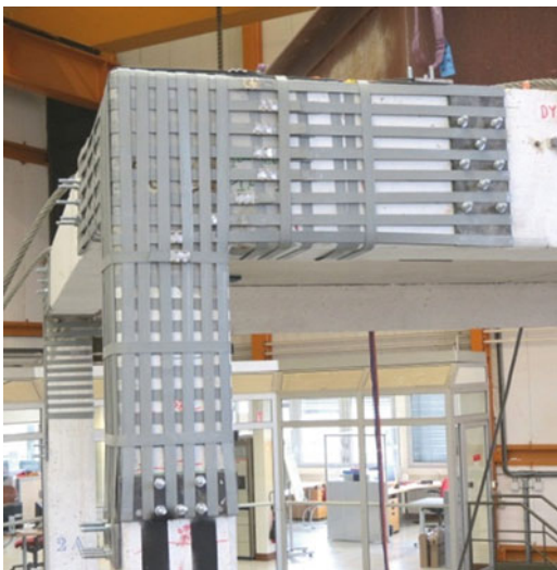
Fig. 11.6 PTMS strengthening at 2nd floor beam-column joints
