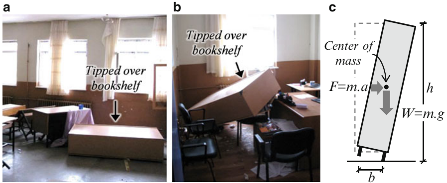
Fig. 3.2 Bookshelves that had tipped over during 2011 M7.2 Van Earthquake: (a) in a typical classroom, and (b) in the director's office, and (c) forces acting on a bookshelf subjected to horizontal acceleration
